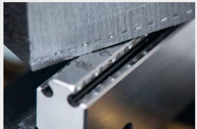
Holding teeth of a Makro·Grip® 5-Axis Vice + stamping contour in workpiece
